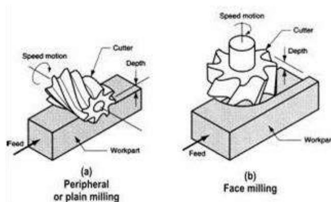
Fig. 1.3 Milling Operations
