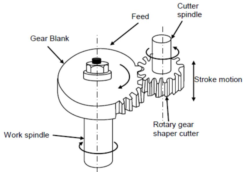
Fig. 1.9(a). Process of Gear Cutting by Shaper Cutter
