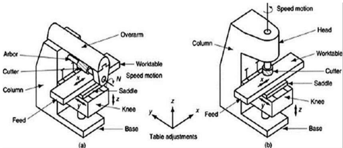
Fig 1.1 Type of Milling Machine
