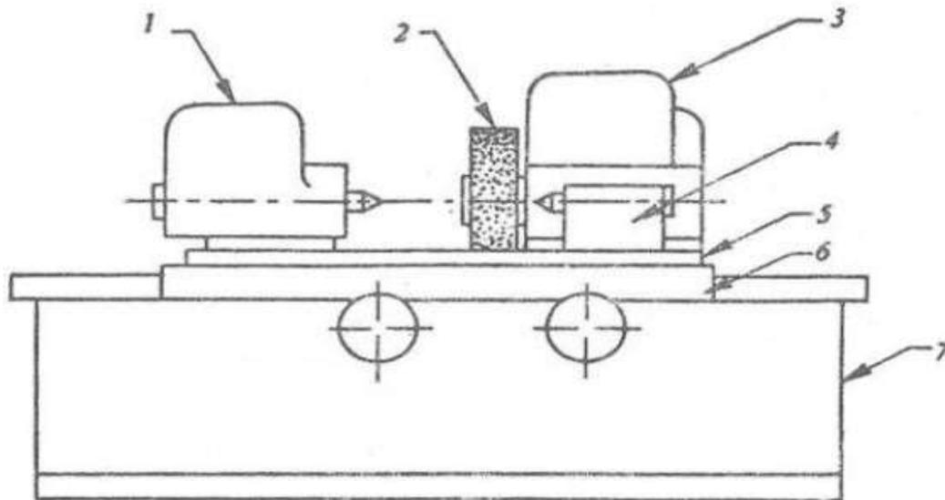
1. Head stock 2. Grinding wheel 3. Wheel head 4. Tail stock 5. Upper table 6. Lower table 7. Base
