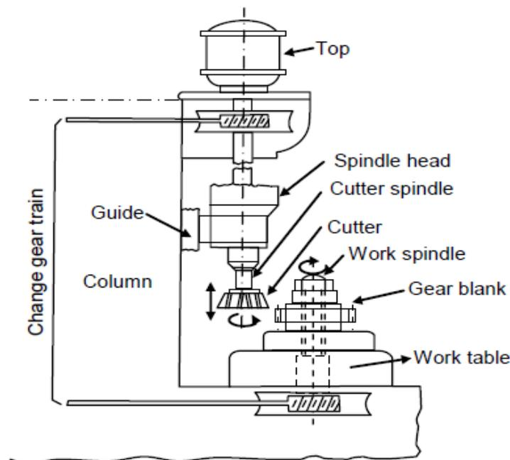
Fig. 1.9(b). Setup for Gear Shaping Machine
