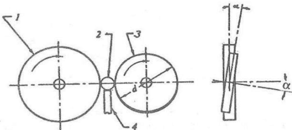
1. Grinding wheel 2. Work 3. Regulating wheel 4. Work rest
