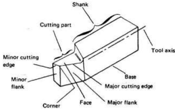
Figure 1.4 Typical single-point tool.
