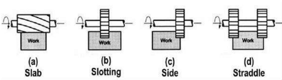
Fig. 1.4 Peripheral Milling
