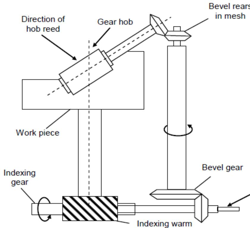
Fig. 2.0 (b). Setup for Gear Hobbing Machine
